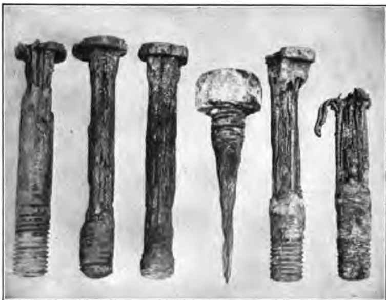
FIG. 4. — Showing the corroded condition of bolts taken from the U. S. Light-Vessel, No. 71.
