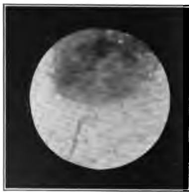
FIG. 57. — Nodule of rust appearing through paint film.
