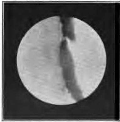
FIG. 48. — Cracking in barytes film and subsequent corrosion showing through.
