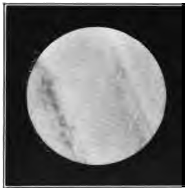
FIG. 55. — Brush marks on paint applied too thick. Thick places liable to break down.
