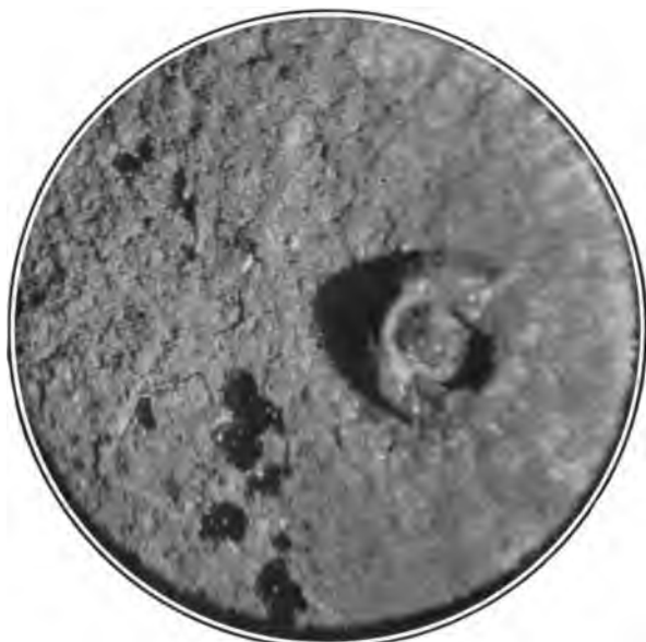
FIG. 15. — Formation of crater with pitting effect in center. (Enlarged 45 diameters.)
