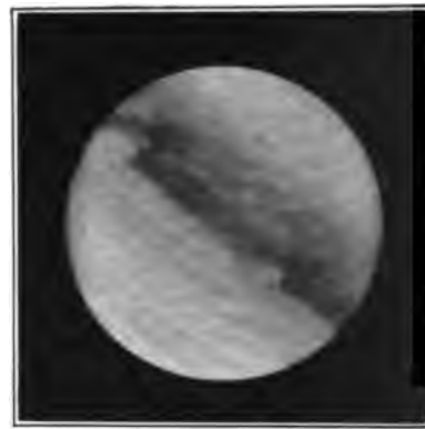
FIG. 52. — Corrosion proceeding from cracks and appearing under surface.
