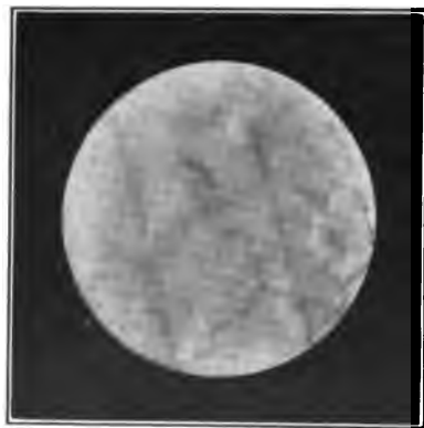
FIG. 54. — Checking of painted surfaces.
