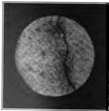
FIG. 56. — Rust exudation on painted panel.
