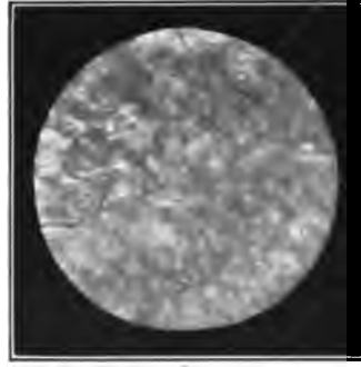
Fig. 45. — Photomicrograph of calcium carbonate. Excessive chalking has caused vehicle decay and rough surface.
